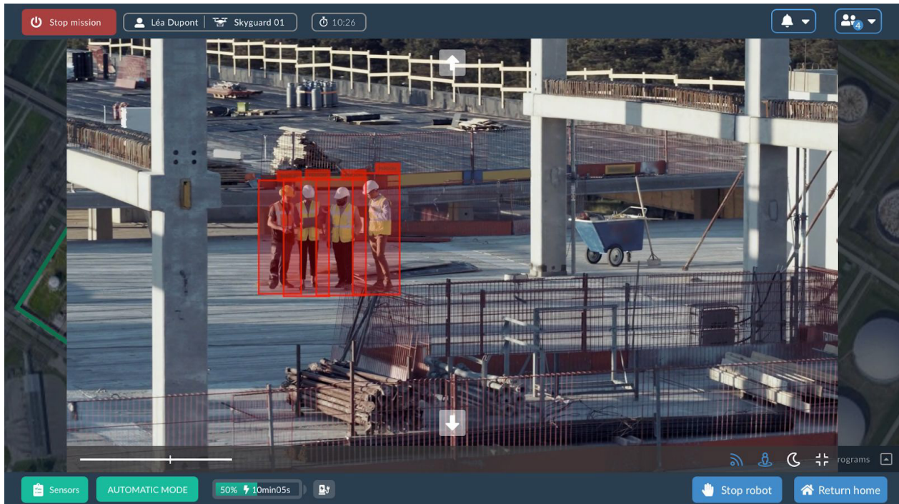
Figure 9: Real-time object detection (workers on a construction site) streamed directly from the drone to UAVIA's web application. All the image processing, drone navigation, and object detection inference are processed in the autonomous drone.
